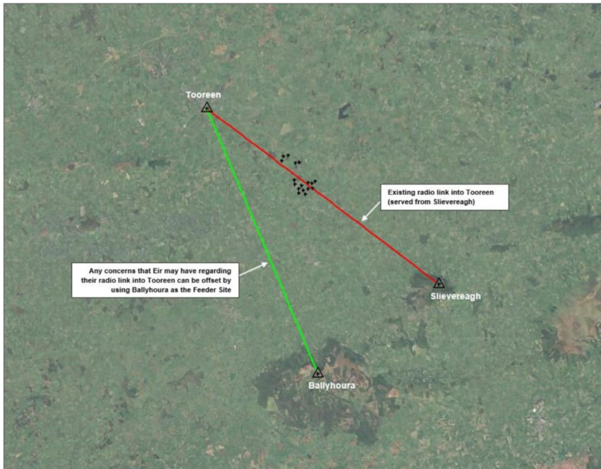
Figure 17-17: Example of how an alternative feeder-site could be used to mitigate against an obstructing turbine
